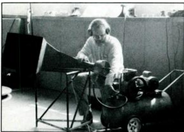
Bruce testing an air powered siren driver.
