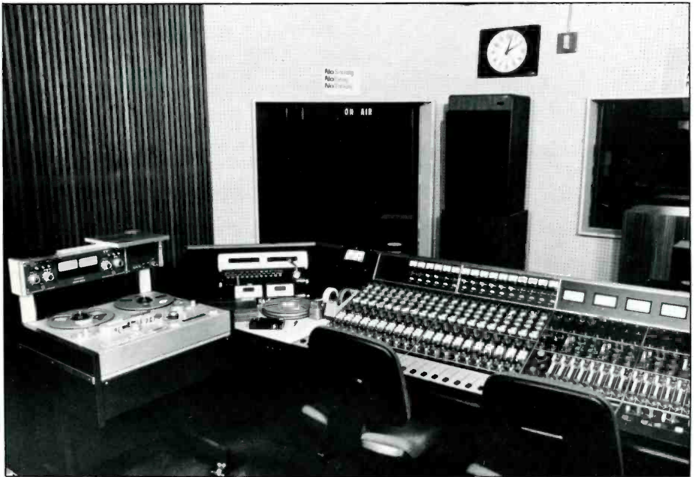
WGBH Control Room One with Neve console and Studer tape machines.
